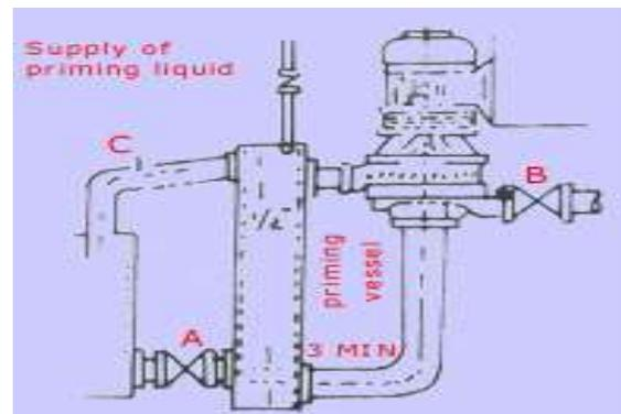
Valve 'A' must be at least 1/2 size large in bore than suction pipe
