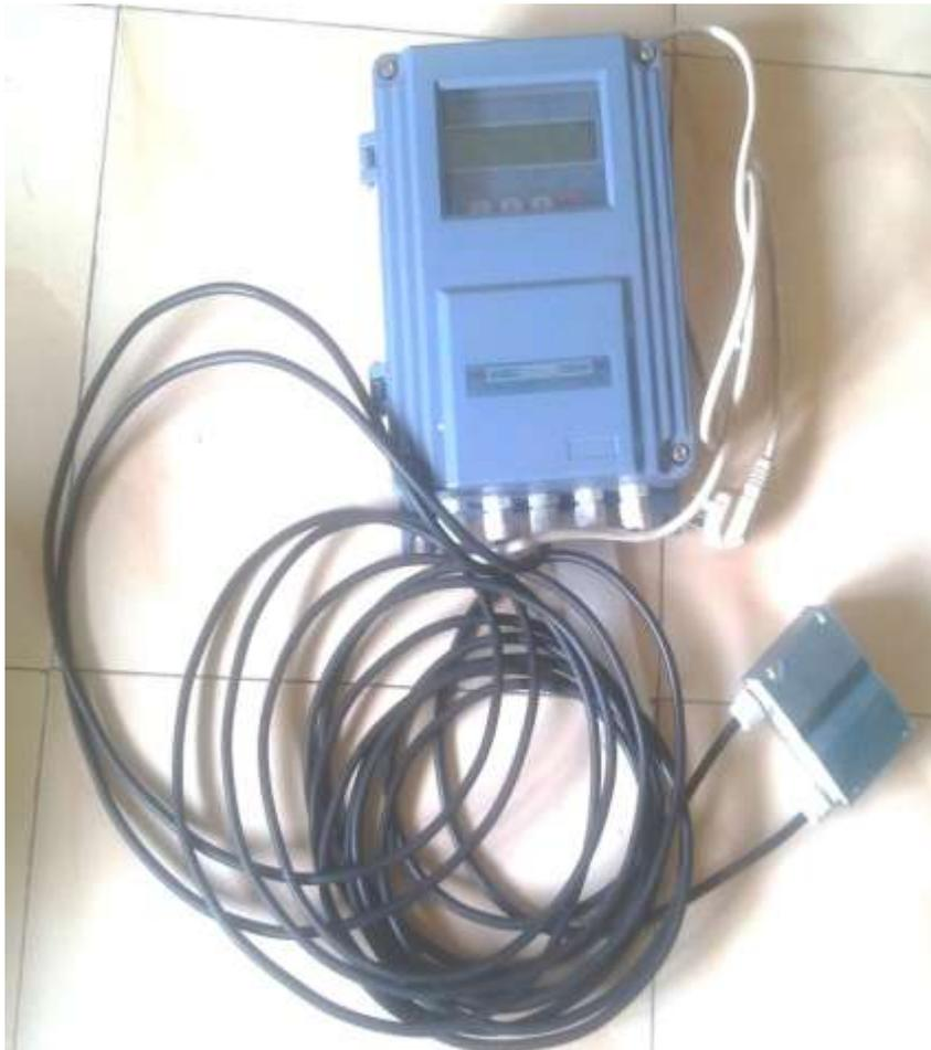
**Fix type ultrasonic flowmeter**
