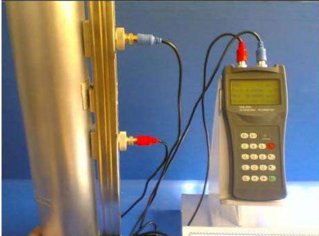
The TDS – 100H Handled Clamp-on Ultrasonic Flow meter is of the most powerful flow meters available for liquid measurement Utilization of our proprietary Ultrasonic Transit-Time measurement and signal quality tracking technologies allow accurate flow measurement of the liquid flow rate from outside of a pipe.
