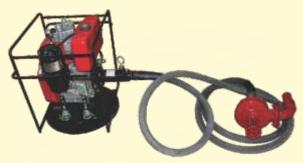
Flexible Shaft Driven Pump can be widely used to handle Dirty water from shallow pit and is also useful to Civil Contractors and Industries to handle water.
