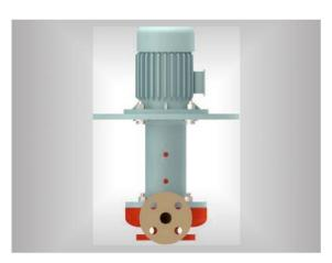
VSP series pumps features a cantilevered FRP sleeved SS316 shaft with key-way in corporate with positive locked Impeller by nut, boxed with single stage volute casing. The unique characteristic of VSP series pumps are that the casing can be rotated for the choice of discharge directions, which adds to the flexibility of installation. Also the suction length flexibility of 300mm & 450mm are available options.
