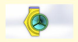
BROIL developed and produced helical rotor flow sensor specially for Liquid dispensing industries, now a day water dispensing industries use plastic turbine flow sensor its k factor change with flow rate so for solution we developer helical rotor plastic flow sensor with same pulse k factor for full range also provide very good accuracy and repeatability in full range of measurement,
